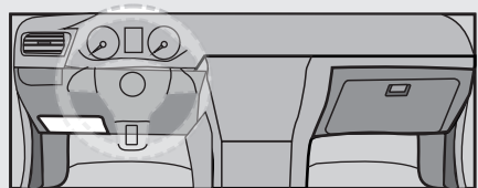
OBD-II connector Front view
