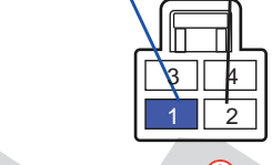
2 Back View White 4-pin connector At brake switch
