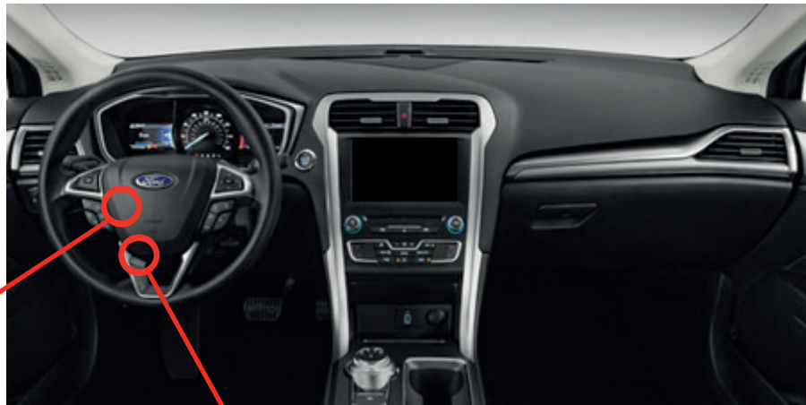
① Gateway module, Behind OBD-II connector
