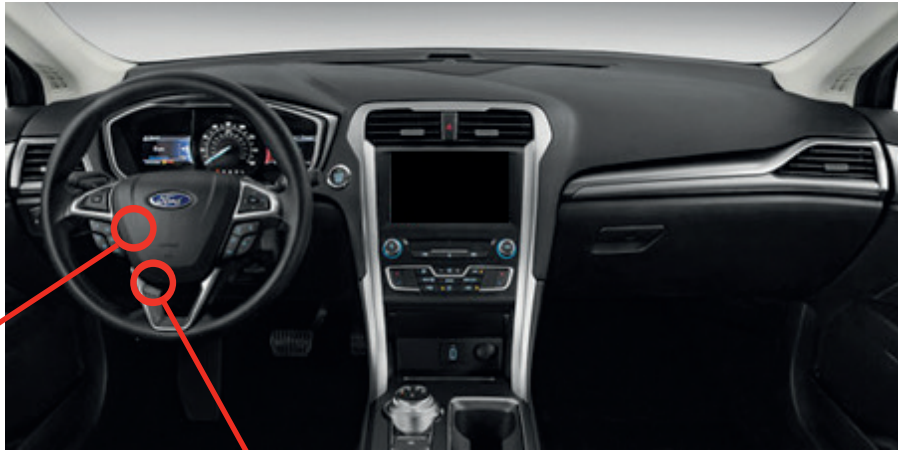
Gateway module, Behind OBD-II connector
