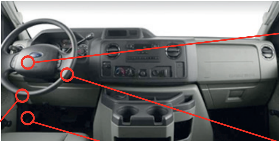
③ Gateway module, Behind OBD-II connector
