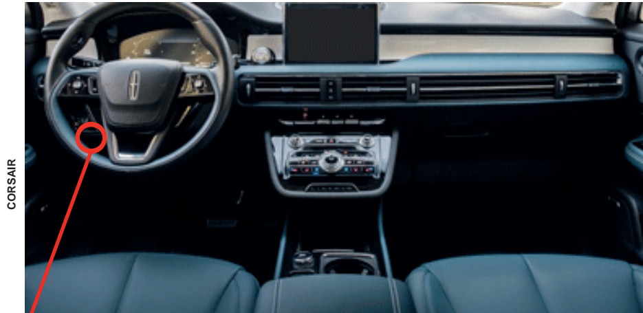
① Gateway module, Behind OBD-II connector
