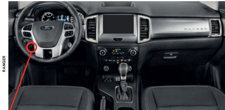
① Gateway module, Behind OBD-II connector
