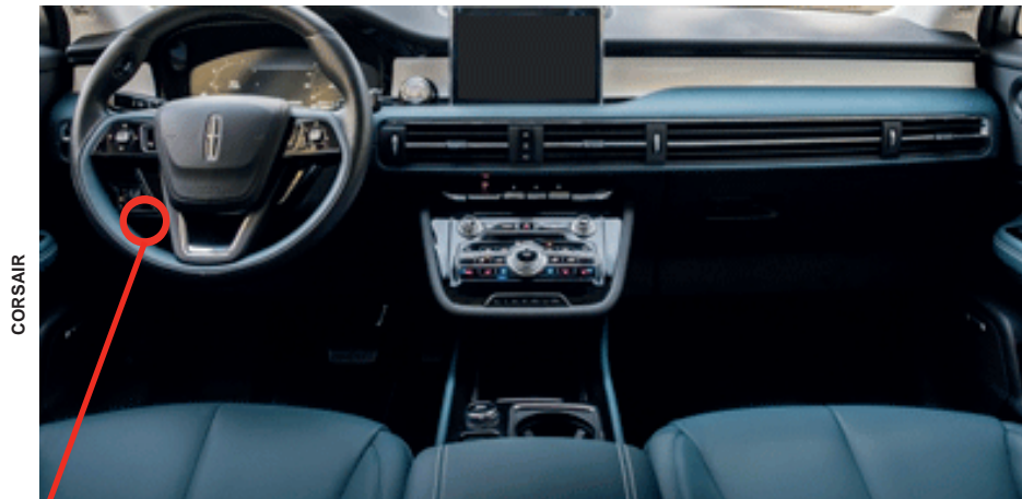
① Gateway module, Behind OBD-II connector
