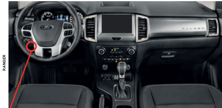
① Gateway module, Behind OBD-II connector
