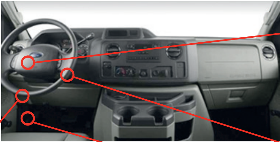
③ Gateway module, Behind OBD-II connector
