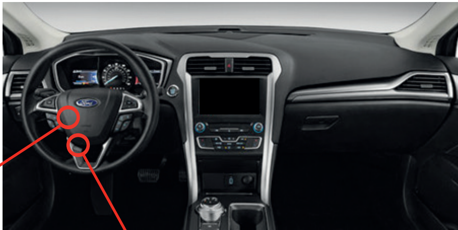
① Gateway module, Behind OBD-II connector
