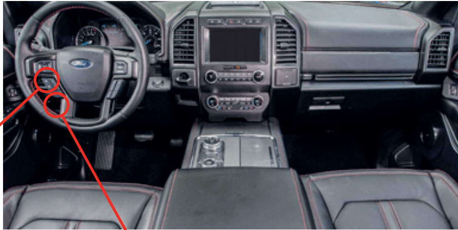
① Gateway module, Behind OBD-II connector
