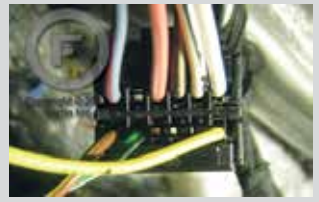
① Back view - Black 12-pin Immobilizer connector, at Ignition barrel.
