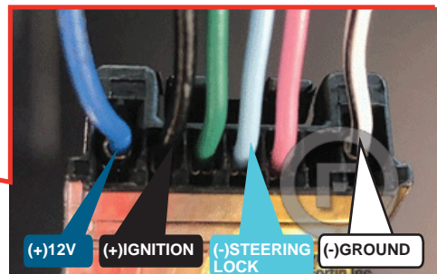
① Steering Lock Connector
