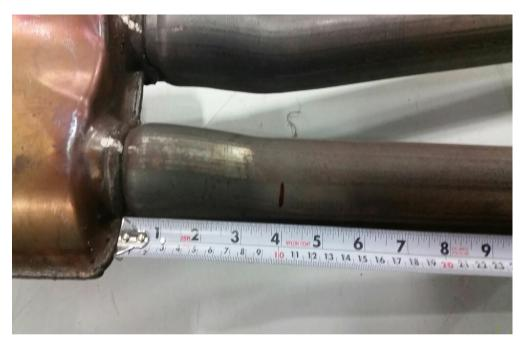
**STEP 6:** Slide the X-pipe into <u>RH</u> catalytic converter and <u>LH</u> muffler inlet pipe clamps. Making sure to center the clamps between the two pipes. Snug both clamps to hold X-pipe in place.
