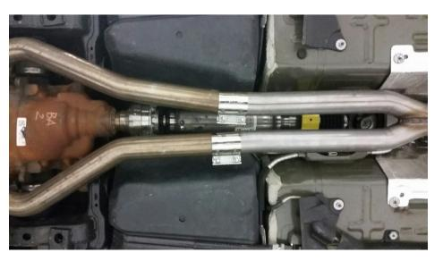
**STEP 9:** Align system in rear facial and torque factory clamps to 35 lb.ft (48 Nm) and the supplied clamps to 40 lb ft (50Nm)
