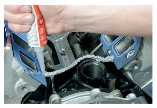
**STEP 13:** Apply a thin layer of silicone around the water openings (4 places).
