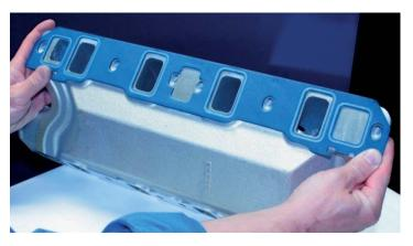
**STEP 2:** Inspect intake manifold for debris, and make sure it's clean. Check all threaded holes and tap deeper if necessary. Check the carburetor/throttle body gasket alignment. Also look at the gasket surfaces for nicks and damage, raised surfaces on the flanges can impede sealing.
