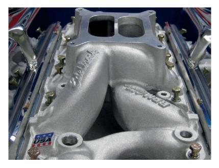
**STEP 16:** Start all bolts by hand and hand tighten. Torque intake manifold bolts in two steps (sequence is shown below):
