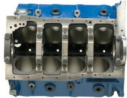
"Using a BOSS 351 block as a foundation became a no-brainer. The block provides about the best bang for the buck anywhere and hardly costs any more than a stock Windsor block that has been fully machined and blueprinted. But the BOSS block still has some advantages over that, namely, it's cast using diesel-grade iron, which exhibits a much greater tensile strength than a stock casting. Plus, there is extra meat in all the critical stress areas.
