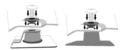
19. Place a Torx head screw through a shoulder washer and into each hole in hood protector. Ensure the shoulder portion of the washer slides into the hole in the hood protector. Loosely thread the screw into the mounting pedestal. See illustration for orientation of the shoulder washer. Repeat for all locations.
