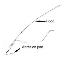
Use one of the surface wipes provided and wipe down the area (approximately 15cm from the hood edge) where the hood protector will be installed. Wipe dry with a soft cloth or paper towel. This will remove any wax or grease and will ensure a cleaner surface for the adhesive to bond to.
