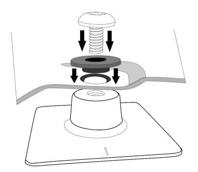
15. Place a Torx head screw through a shoulder washer and into a hole in hood protector. Ensure the shoulder portion of the washer slides into the hole in the hood protector. Loosely thread the screw into the mounting pedestal. See illustration for orientation of the shoulder washer. Repeat for all locations.
