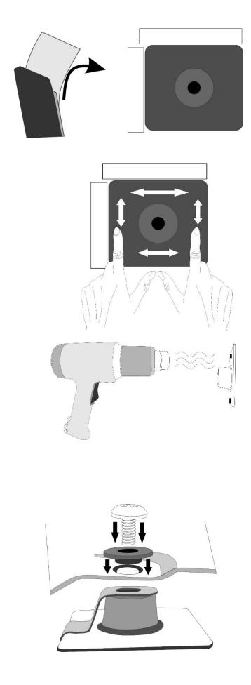
16. Peel the red protective backing off one of the adhesive pedestals. Carefully place it on the hood surface exactly where the tape outline is. Use care with this step as once the pedestal has been placed on the hood, it will be very difficult to remove. Repeat for all locations.
