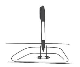
12. Once hood protector is centered, take a felt marker (a fine point Sharpie works best) and insert it into the hole in each of the remaining "pockets" of the hood protector. Keeping the marker perpendicular to the hood surface, mark the hood surface with a dot. \*\*\*NOTE- IF YOUR HOOD HAS PAINT
