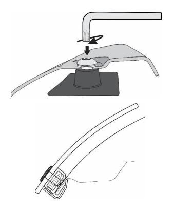
20. Ensure the hood protector is centered on the hood and using a T45 Torx key, tighten the screws into the pedestals. Start in the center position and work outwards. Ensure the shoulder washers are seated properly. Do not overtighten.
