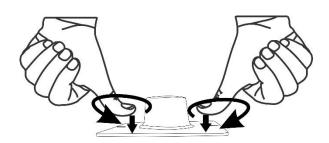
13. To ensure the adhesive is thoroughly bonded to the hood, "wet out" pedestal base by applying pressure with your thumb around the base of the pedestal.
