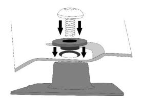
11. Peel the red protective backing off one of the adhesive pedestals. Carefully place it on the hood surface exactly where the tape outline is. Use care with this step as once the pedestal has been placed on the hood, it will be very difficult to remove. Repeat for all locations.
