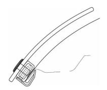
16. Tighten the screws into the hood edge mounting clips.
