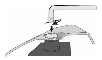
15. Ensure the hood protector is centered on the hood and using a T45 Torx key, tighten the screws into the pedestals. Start in the center position and work outwards. Ensure the shoulder washers are seated properly. Do not overtighten.
