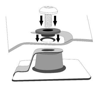
With the hood protector in place, assemble the four pieces of the hood edge clip (see illustrations) and loosely attach it to the edge of the hood. Ensure the hood protector is centered and tighten the screws into the clips.
