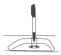
11. Once hood protector is centered, take a felt marker (a fine point Sharpie works best) and insert it into the hole in each of the remaining "pockets" of the hood protector. Keeping the marker perpendicular to the hood surface, mark the hood surface with a dot. \*\*\*NOTE- IF YOUR HOOD HAS PAINT PROTECTION FILM, A PERMANENT MARKER MAY STAIN THE FILM. USE A DRY-ERASE MARKER OR A GREASE PENCIL. \*\*\*
