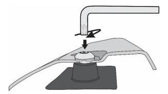
17. Ensure the hood protector is centered on the hood and using a T45 Torx key, tighten the screws into the pedestals. Start in the center position and work outwards. Ensure the shoulder washers are seated properly. Do not overtighten.
