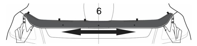
7. If there are tape segments at the front *and* rear of the protector, begin with the rear or trailing edge and centermost tape segment. Hold the tab of the adhesive tape liner and begin removing the liner while applying pressure on the surface of the protector with other hand. See *illustration*. Ensure the tape is well attached by applying firm pressure with your hands on the surface of the protector. Repeat for all tape segments, working away from the center. Repeat this step after 20 min.
