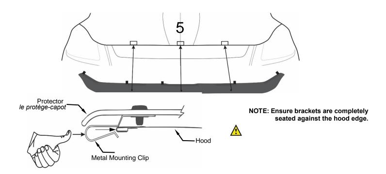
6. Confirm protector is centered on hood visually and by feeling overhang is the same on both ends. Shift protector left or right as required. **Ensure metal brackets remain fully seated**.
