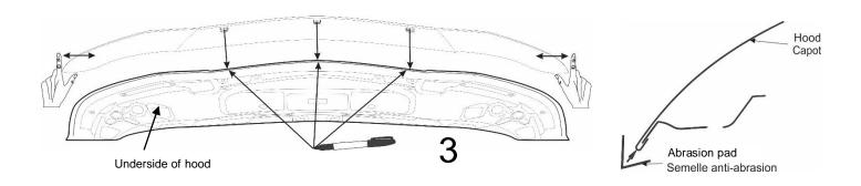
4. Fold tabs on the adhesive tape sections, located on the backside of the protector, so they are accessible after the protector is installed over the edge of the hood. *See illustration*
