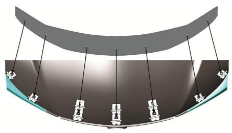
6. Place the hood protector on the pedestals to confirm proper positioning, make any necessary adjustments.
