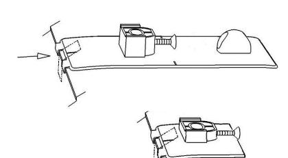
13. Peel and fold the small anti abrasion film pad in half over the hood edge between the fingers on the pedestal.
