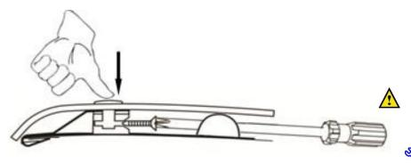
17. Maintain slight pressure on the pin, to ensure proper seating of the components, while simultaneously tightening the screw.
