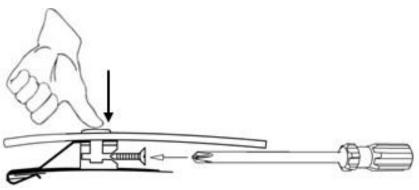
19. Maintain slight pressure on the pin, to ensure proper seating of the components, while simultaneously tightening the screw.
