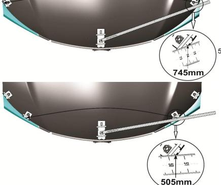
5. Use the center mark on the leading edge of the pedestals for accurate measuring.
