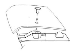
16. At the three (3) large pedestal locations drop a pin through he protector and into the pedestal
