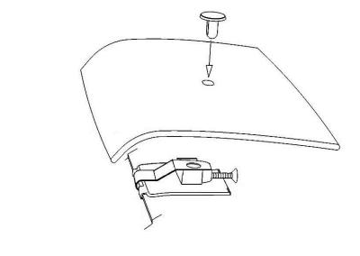
18. At the four (4) small pedestals, drop a pin through the protector and into the pedestal.
