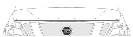
3. Center the "D" gasket laterally on the hood. The "D" gasket installs approximately 1" up from the hood edge. Once its position has been established, peel a small length of the protective backing and place the gasket in position on the hood. Do not peel the full length of backing off! The adhesive is very sticky and once it sticks to something it is very difficult to remove. Peel 3 or 4 inches at a time and press down as you peel.
