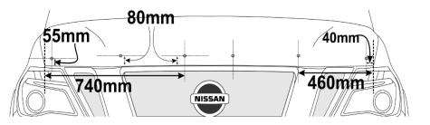
1. Install six (6) bumpons as shown in the diagram below. \*\*Bumpons must be installed on the hood. If they are installed on the hood protector they will wear through the paint on the hood\*\*
