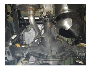
4. Remove nuts (x2) at factory flanged connection behind catalytic converter, separate hangers from isolators on exhaust then remove muffler section. Remove studs (x2) from catalytic converter flange.
