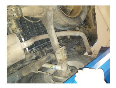
4. Support muffler and disassemble wire hangers from isolators. Remove and retain (x2) bolts and springs from flange then disconnect and remove muffler section from vehicle.
