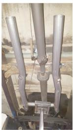
9. Place (x2 ea.) clamps (11) onto mufflers (4) then connect them to h-pipes and tighten clamps enough to allow for later adjustment.
