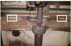
6. Use (x2) rear frame hangers (14) (oriented flanges out) to drill 5%6" mount holes then install hangers with (x2) bolts (15), (x4) flat washers (17), (x2) lock washers (18) and (x2) nuts (16).
