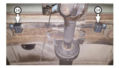
7. Mark rear cross member on both sides, inboard 4" from intersecting frame edge. Use (x2) rear hangers (13) oriented as shown to center then drill mount holes.
