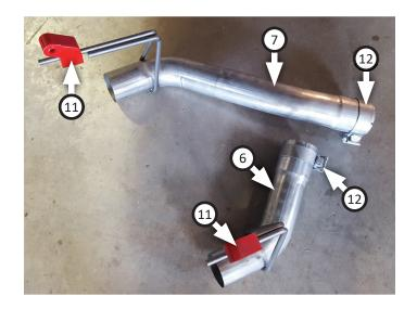
14. Connect right and left rear tailpipes to front tailpipes, then rotate them and to insert hangers. Tighten clamps just enough to allow for later adjustment.
