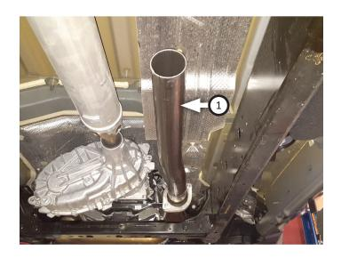
10. Fasten inlet with (x2 ea) bolts (13), flat washers (15), lock washers (16) and nuts (14). Place clamp (12) onto extension (2) and connect it to inlet pipe. Insert hanger in isolator, tighten clamp and reclip ground wire.
