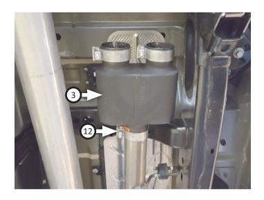
12. Route right front (4) and left front (5) tailpipes over axle then connect them to muffler. Insert their wire hangers into isolators then tighten clamps just enough to allow for adjustment.
