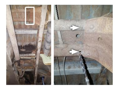
8. Mark line on front crossmember 2<sup>1</sup>/<sub>4</sub>" outward from tank bracket as shown. Use **front frame hanger (12)** oriented as shown to drill (x2) <sup>5</sup>/<sub>16</sub>" mount holes.
