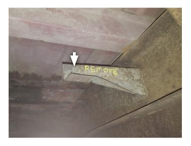
On crossmember above spare tire, make two marks inward from intersecting frame; driver side: 4½" inward, passenger side: 2½" inward. Use (x2) rear hangers (14) oriented as shown to drill (x4) <sup>5</sup>/<sub>16</sub>" mount holes.
