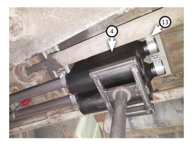
12. Hang (x2) **front hangers (15)** on front of **left (5)** and **right (6)** tailpipes. Hang (x2) rear hangers (step 6) onto rear of left and right tailpipes.
