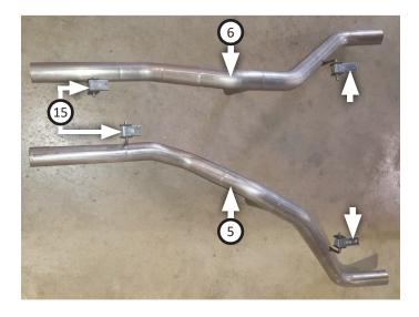
13. Route right tailpipe over axle and connect it to muffler.
