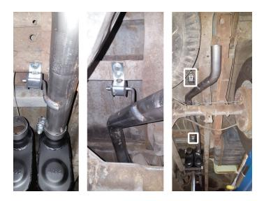
14. Route left tailpipe over axle and connect it to muffler.
