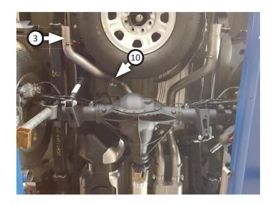
**NOTE:** This kit includes both side and rear exit pipes. A side exit is preferable for towing purposes, to avoid blowing fumes in or on vehicles you may be towing (eg: RV trailer, boat, etc). Otherwise, use **rear exit pipes (6)** in place of side exit pipes.
