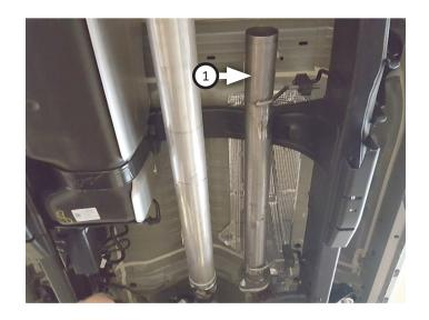
7. Place **clamp (11)** onto **muffler (2)** then connect it to inlet pipe. Tighten clamp just enough to allow for adjustment then place (x2) **clamps (10)** onto muffler outlets.
