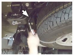
9. Fasten left frame hanger (9) to vehicle using screw (15), backing plate (13), flat washer (16), lock washer (17) and nut (18) as shown. Then hang rubber hanger (12) on frame hanger end.
