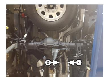
11. Place clamp (10) onto left rear tailpipe (5) then connect it to left front tailpipe. Insert wire hanger into rubber hanger then tighten clamp just enough to allow for later adjustment.
