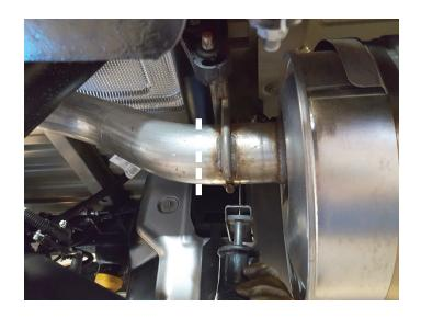
4. Remove nuts (x2) at factory flanged connection behind catalytic converter, separate hangers from isolators on vehicle then remove muffler section. Remove studs (x2) from catalytic converter flange.
