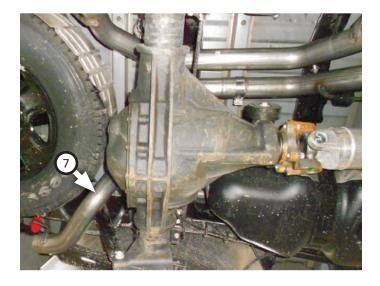
**NOTE:** This kit includes both side and rear exit pipes. A side exit is preferable for towing purposes, to avoid blowing fumes in or on vehicles you may be towing (eg: RV trailer, boat, etc). Otherwise, complete step 13 using **rear exit pipes (9)** in place of side exit pipes.
