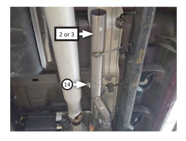
Place clamp (14) onto muffler (4) inlet then connect it to extension pipe. Tighten clamp just enough to allow for adjustment then place clamps (x2) (15) onto muffler outlets.
