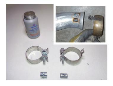
7. Place factory ball clamp (removed step 5) onto **inlet pipe (1)** then connect it to catalytic converter. Insert wire hanger in isolator and tighten clamp enough to allow for adjustment.
