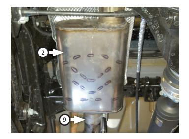
Route y-pipe (3) over rear axle and connect it to muffler, simultaneously inserting wire hanger into isolator.
