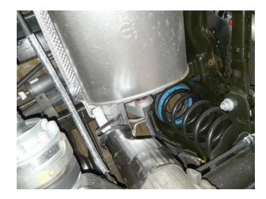
4. Loosen ball clamp, disconnect inlet pipe at catalytic converter and slide exhaust system out and down from vehicle.
