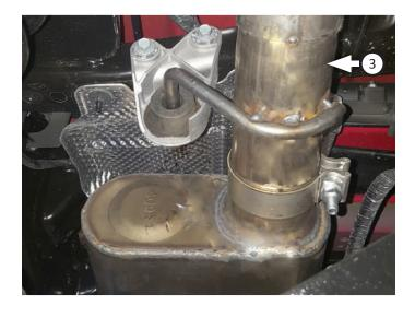
10. Just behind passenger rear tire, unbolt wiring harness bracket. Retain bolts (x2) for later use. Place **clamp (8)** onto **right exit pipe (4)** and connect it to y-pipe right outlet but do not tighten clamp.
