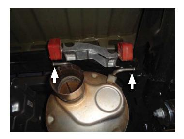
6. Disassemble nuts from factory pipe and catalytic converter flange.
