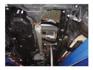
8. Remove stock studs from catalytic converter flange.
