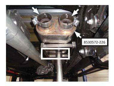
12. Thread **right tailpipe (26729S)** over axle and hang rear wire hanger in stock isolator. Connect right tailpipe to muffler and hang front wire hanger in stock isolator. Tighten clamp just enough to allow for adjustment.
