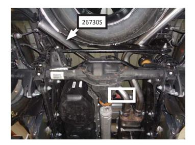
14. Place clamp (MC300BS) onto left exit (26731S) inlet. Connect left exit to left over-axle and hang wire hanger in stock isolator. Tighten clamp just enough to allow for adjustment.
