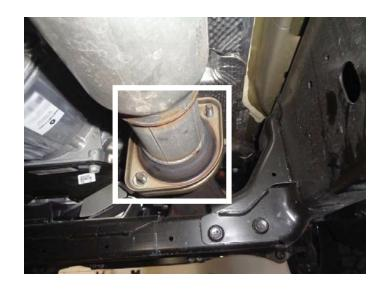
7. Remove muffler and factory pipe from vehicle.
