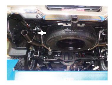
15. Place **tips (x2) (ST462B)** onto left exit and right tailpipe. Tighten nut on tips to fully install them.
