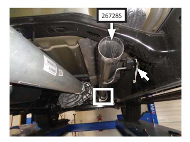
11. Place clamps (x3) (MC300BS) on muffler (8530572-266) inlet and outlets, then connect muffler to inlet pipe.
