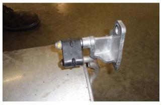
7. Lay the factory and Flowmaster mufflers next to each other, with their inlet pipes pointing the same direction. Then transfer the hanger mounts from the factory muffler to the Flowmaster muffler.
