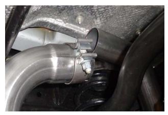
13. Slip a **clamp MC250BS** over the inlet of **muffler 842583-511**. Slide the muffler inlet over the rear of the rear pipe. Support the muffler with a stand, then ensure all pipes are completely seated.
