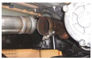
11. Slip the factory clamp over the ball end of the factory pipe, mate the front end of **front pipe 86500S** to it, then snug the clamp just enough to still allow adjustment. Rotate the pipe so that it is level and parallel to the vehicle frame.
