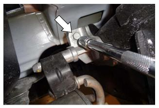
6. Remove each mount's upper bolt. Carefully lower the stand and slide the muffler off of the inlet pipe to remove it from the vehicle.
