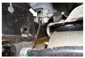
5. At the left and right rear mounts supporting the muffler, remove the lower bolt on each mount.
