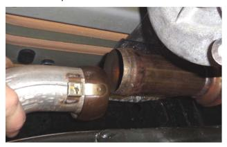
8. Loosen the clamp at the front of the factory midpipe-resonator assembly. Disconnect the hanger on the pipe from the rubber mount on the vehicle and slide the assembly rearward to clear the front cross member, then forward and down to remove it from the vehicle.
