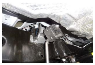
14. Put the factory hanger mounts into position, then reinstall and tighten the factory bolts.
