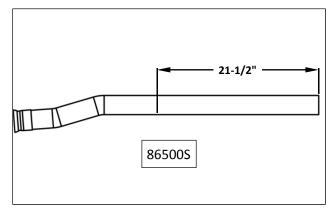
10. FOR TWO-DOOR VEHICLES ONLY, cut 21-1/2" off the rear end of front pipe 86500S.
