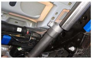
12. Slip a **clamp MC250BS** over the front end of **rear pipe 86501S**, then slide the pipe over the rear of the front pipe while pushing the pipe's hanger into the rubber mount on the vehicle. Snug the clamp just enough to still allow adjustment.
