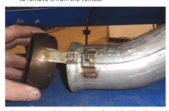
Use a screwdriver to release the tab holding the clamp on the midpipe, and remove the clamp.
