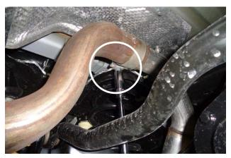
4. Support the muffler with a stand, then loosen the clamp at the muffler inlet connection above the rear axle.
