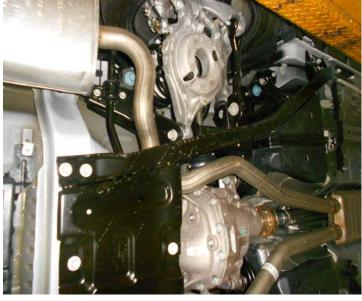
2) On convertible model vehicles, the body braces shown in the photos above will need to be removed in order to remove the factory system and <u>install the Flowmaster system</u>. Starting at the front of the right side (passenger) brace, loosen the front bolt and then work your way to the rear of the vehicle removing the next eight bolts, lower the brace from the vehicle. Repeat this step on the left side of the vehicle with the six bolts on that side.
