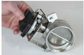
Place a supplied 1/4" Button head screw thru the grounding clip removed from the stock valve and then into the hole on the opposite side of the FM in the mounting plate. Place a supplied ½" spacer between the mount and the actuator heatshield, then follow with a supplied lock washer and nut on the bottom side of the mount.
