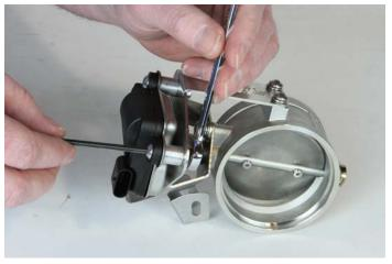
6) Use the remaining  $\frac{1}{4}$ " hardware to secure the actuator to the mount in the remaining two holes. Tighten securely using a 7/16" open end and 5/32" Hex wrench.
