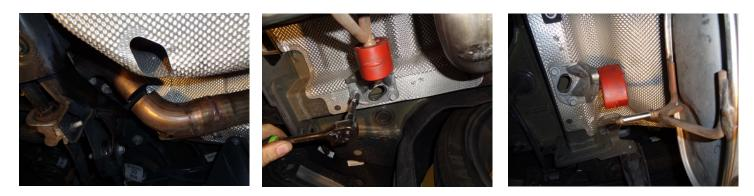
2) To remove the factory exhaust system you will have to cut the system in half. Cutting just before the pipe goes over the rear axle system will allow both halves of the system to be removed easily. After cutting, support the rear muffler with a stand and unbolt the left hanger from the frame. Remove the right hanger on this section from the rubber mount on the vehicle. You can now lower this section from the vehicle.
