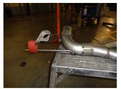
8) Place the left hanger from the factory muffler assembly onto the left hanger rod of exit pipe assembly **#26686S**.
