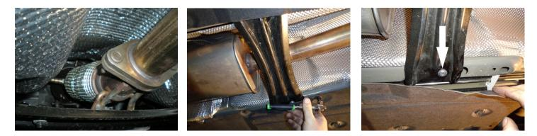
3) In front of the large center muffler, remove the two nuts at the flanged connection just behind the flex joint. Then remove the two bolts from the steel body brace behind the large muffler. Once unbolted, remove the hanger on this section from the rubber mount on the vehicle and lower from the vehicle and set aside. Save the gasket from between the two flanges for use with the Flowmaster system.
