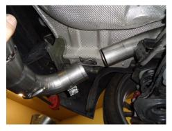
9) Place a supplied clamp onto the front of the exit pipe assembly. Slide the exit pipe assembly over the back of the over-axle pipe and connect the right hanger on the assembly to the rubber mount on the vehicle. Using the factory bolts, reinstall the left hanger back onto the frame of the vehicle. Tighten the clamp enough to hold, but still allow for adjustment.
