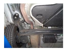
2) To remove the factory exhaust system you will have to cut the system in half. Cutting just before the pipe goes over the rear axle will allow both halves of the system to be removed easily. After cutting, support the rear muffler with a stand and remove the 2 rubber isolators from the mounts on the vehicle, the stock rubber isolators will not be reused. You can now lower this section from the vehicle.
