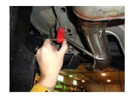
7) Place a supplied clamp onto the inlet of resonator assembly **#15190**. Slide the resonator onto the back of the intermediate pipe and connect the hangers on the assembly to the rubber mounts on the vehicle. Tighten the clamp enough to hold, but still allow for adjustment.
