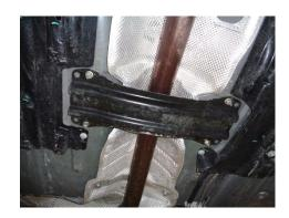
3) In front of the large center muffler, remove the two nuts at the flanged connection just behind the flex joint. Then remove the four nuts from the steel body brace behind the center muffler. Once unbolted, remove the rubber isolators on this section from the mounts on the vehicle and lower from the vehicle and set aside. The stock rubber isolators will not be reused. Save the gasket from between the two flanges for use with the Flowmaster system.
