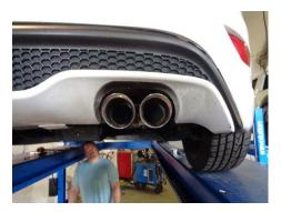
9) Adjust the position of all components to provide a satisfactory fit. This is a tight fitting system, so take your time and be patient, tightening and adjusting a little bit at a time. Be sure to maintain an adequate clearance around all parts of the system to avoid rattles or damage to heat sensitive components. Once you're happy with the fit, tighten all connections down securely. For a cleaner appearance and more secure installation, we highly recommend welding all slip-fit connections.
