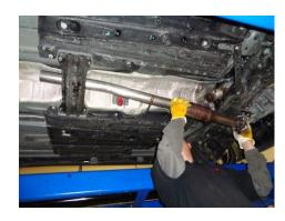
5) Using the nuts removed in step 3 above, bolt muffler assembly **815425-476** to the back of the flex pipe flange. Be sure to replace the gasket. Connect the hangers on the assembly to the rubber mounts on the vehicle and tighten the flanged connection securely. Re-install the steel body brace removed in the previous step and tighten securely.
