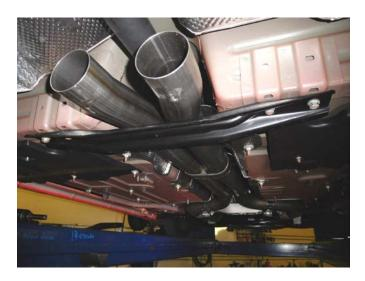
2) Place a supplied 3" clamp onto the inlet neck of both mufflers. Slide the mufflers onto the back of the Scavenger pipe assembly about 1-3/4" and support with stands. Level the mufflers and tighten the clamps enough to hold, but still allow for adjustment.
