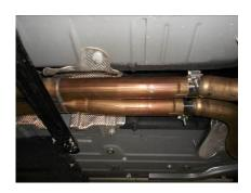
2) Begin by placing a supplied 2 ½" clamp onto each of the slip fits on Scavenger pipe #86337S. Place the Scavenger pipe onto the back of the stock head pipes (make sure the Flowmaster embossing is facing the ground). Level and center the assembly in the drive line tunnel and support with a stand. Tighten the two clamps enough to hold, but still allow for adjustment. Reinstall the two body braces onto the vehicle and tighten securely.
