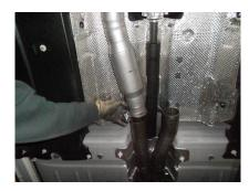
3) Place a supplied 2 ½" clamp onto the inlet of each #815425-460 muffler. Then fully slide the mufflers onto the back of the Scavenger pipe assembly and support with stands. Level the mufflers and tighten the clamps enough to hold, but still allow for adjustment.
