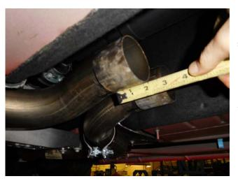
3) Begin the installation by placing a supplied 2-3/4" clamp onto each of the inlets of the Scavenger pipe #26522S. Then place the Scavenger pipe onto the back of the stock head pipes (the offset outlet pipe should be oriented to the passenger side). Level and center the assembly in the drive line tunnel and support with a stand. Scavenger pipe should slide over factory head pipe about 2". Tighten the two clamps enough to hold, but still allow for adjustment.
