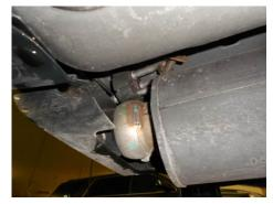
3) Once the factory system is out of the vehicle, use a 5/16 wrench to remove the three nuts securing the actuator to the mounts on the tailpipes. Remove the actuator and spring from the mount on each tailpipe.
