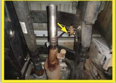
8. Place clamps (MC300BS) (x3) onto inlet and outlets of muffler (8530572-226).
