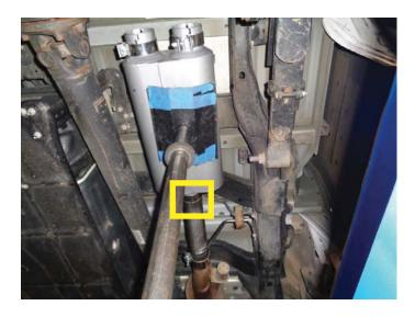
10. Place **right tailpipe (26733S)** into passenger side muffler outlet. Insert both wire hangers into stock mounts to complete connection. Tighten clamp just enough to allow for adjustment.
