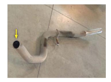
4. Remove muffler hangers (x3) from rubber mounts on vehicle. Loosen clamp at muffler inlet connection.
