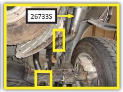
11. Place clamp (MC300BS) onto slip-fit of side exit pipe (26484S). Place side exit pipe into right tailpipe. Tighten clamp just enough to allow for adjustment.
