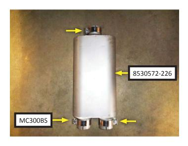
9. Place slip fit of muffler into inlet pipe. Tighten clamp just enough to allow for adjustment.
