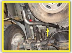
Place clamp (MC300BS) onto slip-fit of side exit pipe (26484S). Connect side exit pipe and left rear tailpipe. Tighten clamp just enough to allow for adjustment.
