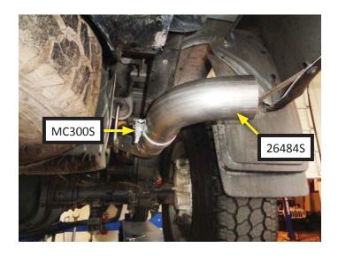
12. Place **left front tailpipe (26734S),** into driver side muffler outlet. Insert wire hanger into stock mount. Tighten clamp just enough to allow for adjustment.
