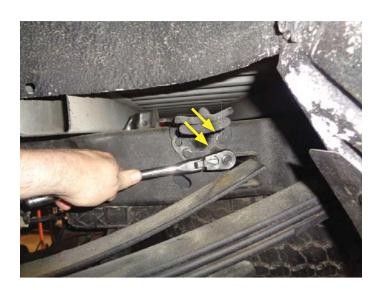
14. Place hanger (503HA) onto vehicle frame then reinstall factory bolts (x2) (removed step 13). Install isolator (HA168) onto hanger.
