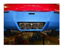
1) Before you begin, please understand that the installation of this system requires significant disassembly. The entire lower rear bumper fascia (Blue portion in photo) must be removed. Because this is a painted body panel, you may want to consider covering it with masking tape for the disassembly/assembly process to prevent any scratches. Note: Do not turn the vehicle ignition on anytime during the removal/assembly process
