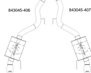
Description Qty Part# 1 Left Muffler Assembly. 843045-406 Right Muffler Assembly. 843045-407 1
