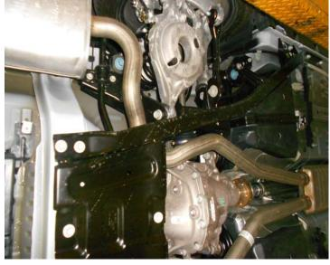
On convertible model vehicles, the body braces show in the photos above will need to be removed in order remove the factory system and install the Flowmaster system. Starting at the front of the right side (passenger) brace, loosen the front bolt and then work your way to the rear of the vehicle removing the next eight bolts, lower the brace from the vehicle. Repeat this step on the left side of the vehicle with the six bolts on that side.
