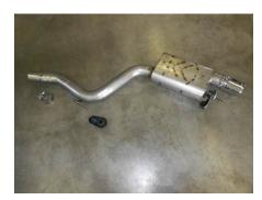
1) Place the new Flowmaster muffler units next to the factory units and swap the front and rear hanger mounts from the stock mufflers to the Flowmaster assemblies. Also, place a provided 2.25" clamp onto the inlet of each assembly. Tighten the clamp just enough to hold in place.
