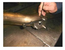
2) Then mount with the spacers and washers attached. Tighten securely.
