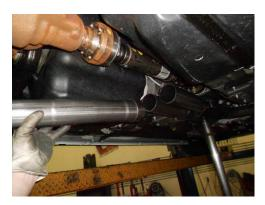
2) Place a provided 3" clamp onto the expanded end of left mid pipe **#26514S**, then slide completely onto the left side of the Scavenger assembly and tighten the clamp enough to hold, but still allow for adjustment. Repeat this step on the right side of the vehicle with mid pipe **#26515S**.
