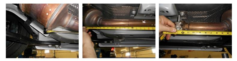
4) Begin by measuring back 11" from the bottom case weld on both catalytic converters as shown in the photos above and make a mark on both pipes. Support the exhaust system behind the area to be cut, then once you've double checked that the measurements are correct, cut both pipes at the marks. **Note: Due to the closeness of the pipes to the floor of the vehicle, use caution when cutting!** Carefully deburr the end of the pipes where cut with a file or die grinder.
