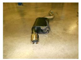
3) Place the new Flowmaster muffler units next to the factory exhaust system and swap the front and rear hanger mounts from the stock mufflers to the Flowmaster assemblies. Also, place a provided 3.00" clamp onto the inlet of each muffler assembly. Tighten the clamp just enough to hold in place.
