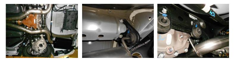
4) Place the right muffler assembly **#853067-389** up into position and slide the inlet completely onto the **26515S** mid pipe. Support the assembly with a stand and remount the rear hanger mount to the frame, tighten securely. Remount the front hanger to the cross member and tighten securely. Leave the clamp on the inlet loose for now. Repeat this step with muffler assembly **#853067-388** on the left side of the vehicle.
