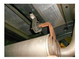
2) Begin by applying a lubricant to each of the rubber exhaust isolators as well as the two front flange bolts. This will make the removal and installation process much easier.
