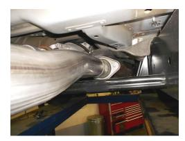
3) Place the inlet pipe onto the back of the existing OEM head pipe and fasten using the 3/8" x 2.00" bolts, nuts and washers provided in the hardware kit. Tighten just enough to hold in place, but still allow for adjustment.
