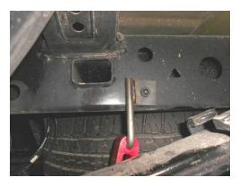
1) Mount the left rear tailpipe hanger bracket **#226HA** to the frame on the driver's side of the vehicle. Place the included 3/8 x 3.50" bolt thru the 226HA hanger and into the hole indicated in the photo. On the inside of the frame, place the HA226 back-up plate over the bolt followed by a flat washer, lock washer and nut. Using two 9/16" wrenches tighten firmly (Do not over tighten).
