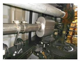
4) Slide the inlet hanger #490HA over the back of the inlet pipe and insert the hanger into the factory rubber mount. Do not tighten this clamp yet. If required, place the extension pipe #26277S onto the back of the inlet pipe. Then place the inlet of the muffler onto the back of inlet pipe and support with a stand. Level the muffler and tighten the clamp at the inlet enough to hold, but still allow for adjustment.
