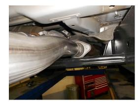
3) Place the inlet pipe onto the back of the existing OEM head pipe and fasten using the 3/8" x 2.00" bolts, nuts and washers provided in the hardware kit. Tighten just enough to hold in place, but still allow for adjustment.
