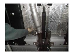
2) Place a supplied 3" clamp onto the inlet neck of both mufflers. Slide the mufflers onto the back of the Scavenger pipe assembly and support with stands. Level the mufflers and tighten the clamps enough to hold, but still allow for adjustment.
