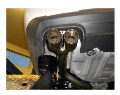
3) Place a supplied clamp onto the left muffler outlet. Place the left tailpipe **#26530S** into position and starting from the rear, connect the hangers on the tailpipe to the rubber mounts on the vehicle. Slide the tailpipe fully into the muffler outlet. Adjust the tailpipe so that the stainless tip is level and centered in the bumper cut-out. Tighten clamp enough to hold, but still allow for adjustment. Repeat this step for right tailpipe **#26531S**.
