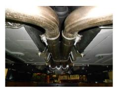
1) Begin the installation by placing a supplied 2-1/2" clamp onto each of the inlets of the Scavenger assembly **#26528S**. Then place the Scavenger pipe onto the back of the stock head pipes (the offset outlet pipe should be oriented to the passenger side). Level and center the assembly in the drive line tunnel and support with a stand. Tighten the two clamps enough to hold, but still allow for adjustment.
