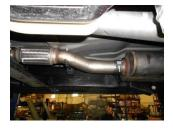
5) Place the provided 3" clamp onto the inlet of muffler **#853057-Z**, then connect the inlet of the muffler to the inlet pipe and support with a stand. Tighten the clamp just enough to hold in position.
