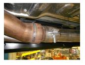
4) Trim inlet pipe **#26428S** according to the following measurements before placing onto the stock front pipe just behind the catalytic converter. Be sure to line up the notch in the pipe with the tab on the front pipe. Place the provided 3" clamp onto this connection and tighten enough to hold.
