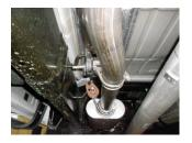
5) Slide clamp hanger **#459HA** over the back of inlet pipe **#26428S** and connect to the rubber mount on the frame located midway between the converter and the muffler.
