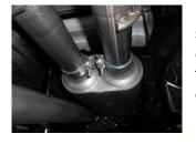
9) Install a provided 2½" clamp onto the left muffler outlet. Place the front section of the left side tailpipe **#86194S** into the left side muffler outlet and connect the hanger on the pipe to the rubber mount on the vehicle. Tighten the clamp enough to hold, but still allow for adjustment. Place a second 2½" onto the back of this pipe in preparation for the next step.
