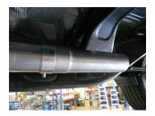
2) If installing the system on a Crew Cab truck with a 6.5' bed, place extension pipe **#TB700S** onto the back of the **#26429S** inlet pipe, place a provided clamp onto the slip-fit and tighten enough to hold in position. This extension pipe will not be used on Double Cab or Crew Cab-5.5' bed models.
