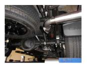
7) Slide the side exit pipes **#26433S** or the rear exit pipes **#26454S** onto the ends of both over axle pipes and place a supplied 2-1/2" clamp onto these slip-fit connections. Tighten just enough to hold in position. Place the two stainless tips **#ST462B** onto the exit pipes and tighten them enough to hold position. Rotate the exit pipes and tips to the desired distance from the body or bumper, so that the angle cut on the tips are in the desired location.
