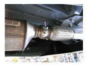
1) Place inlet pipe assembly #26453S into position onto the ball connection behind the catalytic converter. Reinstall the clamp onto the ball connection and tighten enough to hold, but still allow for a small amount of adjustment. Rotate the pipe so that the rear of the pipe is positioned up toward the floor of the truck. Support the rear of the pipe with a stand.
