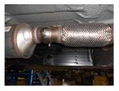
4) 2009-13 Models: Using a 15mm wrench, loosen the bolt on the clamped ball connection behind the catalytic converter. Separate the wire hangers from the rubber mounts on the vehicle and lower the inlet pipe and muffler from the vehicle. You will need to remove the ball clamp from the stock system; it will be reused with the Flowmaster system.
