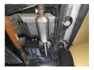
2) Place a provided clamp onto the inlet of muffler **#12518409-Z** and slide over the back of inlet pipe **#710TBS**. Tighten the clamp enough to hold, but still allow for adjustment.
